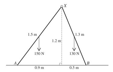
Two uniform rods XA and XB are freely jointed at X. The lengths of the rods are 1.5 m and 1.3 m respectively, and their weights are 150 N and 130 N respectively. The rods are in equilibrium in a vertical plane with A and B in contact with a rough horizontal surface. A and B are at distances horizontally from X of 0.9 m and 0.5 m respectively, and X is 1.2 m above the surface (see diagram).
