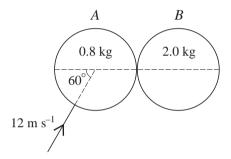
Two uniform smooth spheres A and B, of equal radius, have masses  $0.8 \,\mathrm{kg}$  and  $2.0 \,\mathrm{kg}$  respectively. The spheres are on a horizontal surface. A is moving with speed  $12 \,\mathrm{m\,s^{-1}}$  at  $60^{\circ}$  to the line of centres when it collides with B, which is stationary (see diagram). The coefficient of restitution between the spheres is 0.75. Find the speed and direction of motion of A immediately after the collision. [10]
