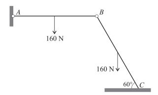
Two identical uniform rods, AB and BC, are freely jointed to each other at B, and A is freely jointed to a fixed point. The rods are in limiting equilibrium in a vertical plane, with C resting on a rough horizontal surface. AB is horizontal, and BC is inclined at  $60^{\circ}$  to the horizontal. The weight of each rod is  $160 \,\mathrm{N}$  (see diagram).
