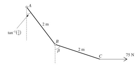
Two uniform rods AB and BC, each of length 2 m, are freely jointed at B. The weights of the rods are W N and 50 N respectively. The end A of AB is hinged at a fixed point. The rods AB and BC make angles  $\tan^{-1}\left(\frac{3}{4}\right)$  and  $\beta$  respectively with the downward vertical, and are held in equilibrium in a vertical plane by a horizontal force of magnitude 75 N acting at C (see diagram).
