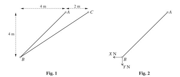
Two uniform rods AB and BC, of weights 70 N and 110 N respectively, are freely jointed at B. The rods are in equilibrium in a vertical plane with A and C at the same horizontal level and AC = 2 m. The rod AB is freely jointed to a fixed point at A and the rod BC is freely jointed to a fixed point at C. The horizontal distance between B and A is 4 m and B is 4 m below AC; angle BAC is obtuse (see Fig. 1). The force exerted on the rod AB at B, by the rod BC, has horizontal and vertical components
