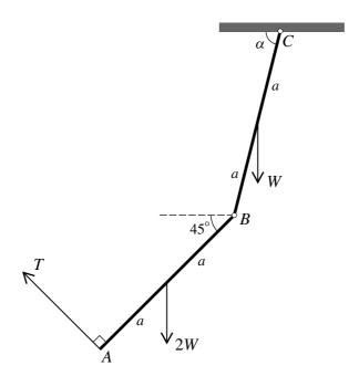
Two uniform rods AB and BC, each of length 2a, have weights 2W and W respectively. The rods are freely jointed to each other at B, and BC is freely jointed to a fixed point at C. The rods are held in equilibrium in a vertical plane by a light string attached to A and perpendicular to AB. The rods AB and BC make angles  $45^{\circ}$  and  $\alpha$ , respectively, with the horizontal. The tension in the string is T (see diagram).
