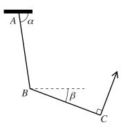
Two uniform rods AB and BC, each of length 2Lm and of weight 84.5 N, are freely jointed at B, and AB is freely jointed to a fixed point at A. The rods are held in equilibrium in a vertical plane by a light string attached at C and perpendicular to BC. The rods AB and BC make angles  $\alpha$  and  $\beta$  to the horizontal, respectively (see diagram). It is given that  $\cos \beta = \frac{12}{13}$ .
