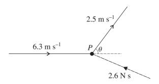
A particle P of mass 0.5 kg is moving in a straight line with speed 6.3 m s<sup>-1</sup>. An impulse of magnitude 2.6 N s applied to P deflects its direction of motion through an angle  $\theta$ , and reduces its speed to 2.5 m s<sup>-1</sup> (see diagram). By considering an impulse-momentum triangle, or otherwise,
