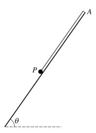
A particle P, of mass 3.5 kg, is in equilibrium suspended from the top A of a smooth slope inclined at an angle  $\theta$  to the horizontal, where  $\sin \theta = \frac{40}{49}$ , by an elastic rope of natural length 4 m and modulus of elasticity 112 N (see diagram). Another particle Q, of mass 0.5 kg, is released from rest at A and slides freely downwards until it reaches P and becomes attached to it.
