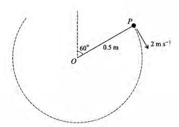
One end of a light inextensible string of length 0.5 m is attached to a fixed point O. A particle P of mass 0.3 kg is attached to the other end of the string. With the string taut and at an angle of  $60^{\circ}$  to the upward vertical, P is projected with speed  $2 \,\mathrm{m\,s^{-1}}$  (see diagram). P begins to move without air resistance in a vertical circle with centre O. When the string makes an angle  $\theta$  with the upward vertical, the speed of P is  $v \,\mathrm{m\,s^{-1}}$ .
