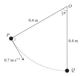
A particle P of mass 0.8 kg is attached to a fixed point O by a light inextensible string of length 0.4 m. A particle Q is suspended from O by an identical string. With the string OP taut and inclined at  $\frac{1}{3}\pi$  radians to the vertical, P is projected with speed 0.7 m s<sup>-1</sup> in a direction perpendicular to the string so as to strike Q directly (see diagram). The coefficient of restitution between P and Q is  $\frac{1}{7}$ .
