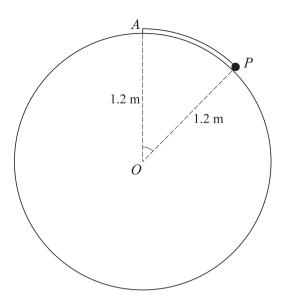
The diagram shows a particle *P* of mass 0.5 kg attached to the highest point *A* of a fixed smooth sphere by a light elastic string. The sphere has centre *O* and radius 1.2 m. The string has natural length 0.6 m and modulus of elasticity 6.86 N. *P* is released from rest at a point on the surface of the sphere where the acute angle *AOP* is at least 0.5 radians.
