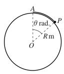
One end of a light elastic string, of natural length  $\frac{2}{3}R$  m and with modulus of elasticity 1.2mg N, is attached to the highest point A of a smooth fixed sphere with centre O and radius R m. A particle P of mass mkg is attached to the other end of the string and is in contact with the surface of the sphere, where the angle AOP is equal to  $\theta$  radians (see diagram).
