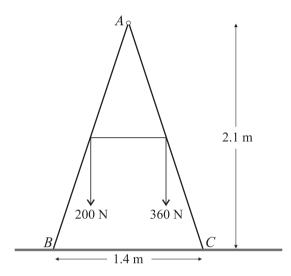
Two uniform rods AB and AC, of equal lengths, and of weights 200 N and 360 N respectively, are freely jointed at A. The mid-points of the rods are joined by a taut light inextensible string. The rods are in equilibrium in a vertical plane with B and C in contact with a smooth horizontal surface. The point A is 2.1 m above the surface and BC = 1.4 m (see diagram).
