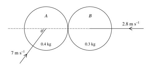
Two uniform smooth spheres A and B of equal radius are moving on a horizontal surface when they collide. A has mass 0.4 kg and B has mass 0.3 kg. Immediately before the collision A is moving with speed  $7 \,\mathrm{m \, s^{-1}}$  at an acute angle  $\theta$  to the line of centres, where  $\cos \theta = 0.6$ , and B is moving with speed  $2.8 \,\mathrm{m \, s^{-1}}$  along the line of centres (see diagram). The coefficient of restitution between the spheres is 0.7. Find
