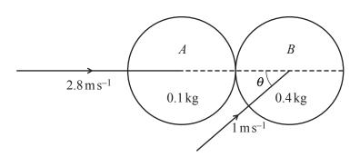
Two uniform smooth spheres A and B of equal radius are moving on a horizontal surface when they collide. A has mass 0.1 kg and B has mass 0.4 kg. Immediately before the collision A is moving with speed  $2.8 \,\mathrm{m\,s^{-1}}$  along the line of centres, and B is moving with speed  $1 \,\mathrm{m\,s^{-1}}$  at an angle  $\theta$  to the line of centres, where  $\cos \theta = 0.8$  (see diagram). Immediately after the collision A is stationary. Find
