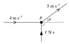
A particle P of mass 0.3 kg is moving in a straight line with speed  $4 \,\mathrm{m\,s^{-1}}$  when it is deflected through an angle  $\theta$  by an impulse of magnitude  $I \,\mathrm{N\,s}$ . The impulse acts at right angles to the initial direction of motion of P (see diagram). The speed of P immediately after the impulse acts is  $5 \,\mathrm{m\,s^{-1}}$ . Show that  $\cos \theta = 0.8$  and find the value of I.
