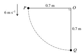
A particle P is attached to a fixed point O by a light inextensible string of length 0.7 m. A particle Q is in equilibrium suspended from O by an identical string. With the string OP taut and horizontal, P is projected vertically downwards with speed  $6 \,\mathrm{m\,s^{-1}}$  so that it strikes Q directly (see diagram). P is brought to rest by the collision and Q starts to move with speed  $4.9 \,\mathrm{m\,s^{-1}}$ .
