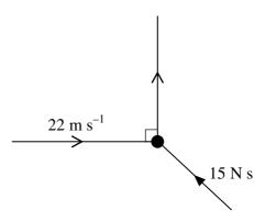
A ball of mass  $0.5 \,\mathrm{kg}$  is moving with speed  $22 \,\mathrm{m\,s^{-1}}$  in a straight line when it is struck by a bat. The impulse exerted by the bat has magnitude  $15 \,\mathrm{N\,s}$  and the ball is deflected through an angle of  $90^\circ$  (see diagram). Find
