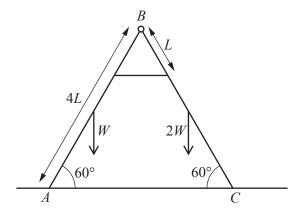
Two uniform rods AB and BC, each of length 4L, are freely jointed at B, and rest in a vertical plane with A and C on a smooth horizontal surface. The weight of AB is W and the weight of BC is 2W. The rods are joined by a horizontal light inextensible string fixed to each rod at a point distance L from B, so that each rod is inclined at an angle of  $60^{\circ}$  to the horizontal (see diagram).
