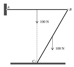
Two uniform rods AB and BC are of equal length and each has weight 100 N. The rods are freely jointed to each other at B, and A is freely jointed to a fixed point. The rods are in equilibrium in a vertical plane with AB horizontal and C resting on a rough horizontal surface. C is vertically below the mid-point of AB (see diagram).
