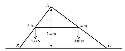
Two uniform rods AB and AC, of lengths 3 m and 4 m respectively, have weights 300 N and 400 N respectively. The rods are freely jointed at A. The mid-points of the rods are joined by a light inextensible string. The rods are in equilibrium in a vertical plane with the string taut and B and C in contact with a smooth horizontal surface. The point A is 2.4 m above the surface (see diagram).
