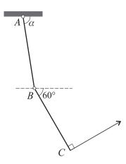
Two uniform rods AB and BC, each of length 1.4 m and weight 80 N, are freely jointed to each other at B, and AB is freely jointed to a fixed point at A. They are held in equilibrium with AB at an angle  $\alpha$  to the horizontal, and BC at an angle of  $60^{\circ}$  to the horizontal, by a light string, perpendicular to BC, attached to C (see diagram).
