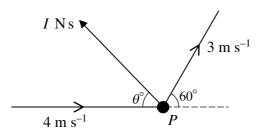
A particle P of mass 0.4 kg is moving horizontally with speed  $4 \,\mathrm{m\,s^{-1}}$  when it receives an impulse of magnitude  $I \,\mathrm{N}\,\mathrm{s}$ , in a direction which makes an angle  $(180 - \theta)^\circ$  with the direction of motion of P. Immediately after the impulse acts P moves horizontally with speed  $3 \,\mathrm{m\,s^{-1}}$ . The direction of motion of P is turned through an angle of  $60^\circ$  by the impulse (see diagram). Find I and  $\theta$ .
