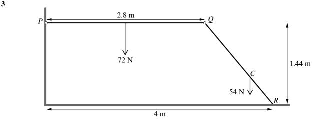
A uniform rod PQ has weight 72 N. A non-uniform rod QR has weight 54 N and its centre of mass is at C, where QC = 2CR. The rods are freely jointed to each other at Q. The rod PQ is freely jointed to a fixed point of a vertical wall at P and the rod QR rests on horizontal ground at R. The rod PQ is 2.8 m long and is horizontal. The point R is 1.44 m below the level of PQ and 4 m from the wall (see diagram).
