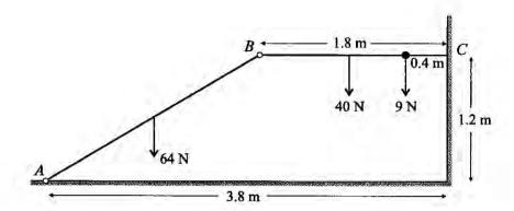
Two uniform rods AB and BC have weights 64 N and 40 N respectively. The rods are freely jointed to each other at B. The rod AB is freely jointed to a fixed point on horizontal ground at A and the rod BC rests against a vertical wall at C. The rod BC is 1.8 m long and is horizontal. A particle of weight 9 N is attached to the rod BC at the point 0.4 m from C. The point A is 1.2 m below the level of BC and 3.8 m from the wall (see diagram). The system is in equilibrium.
